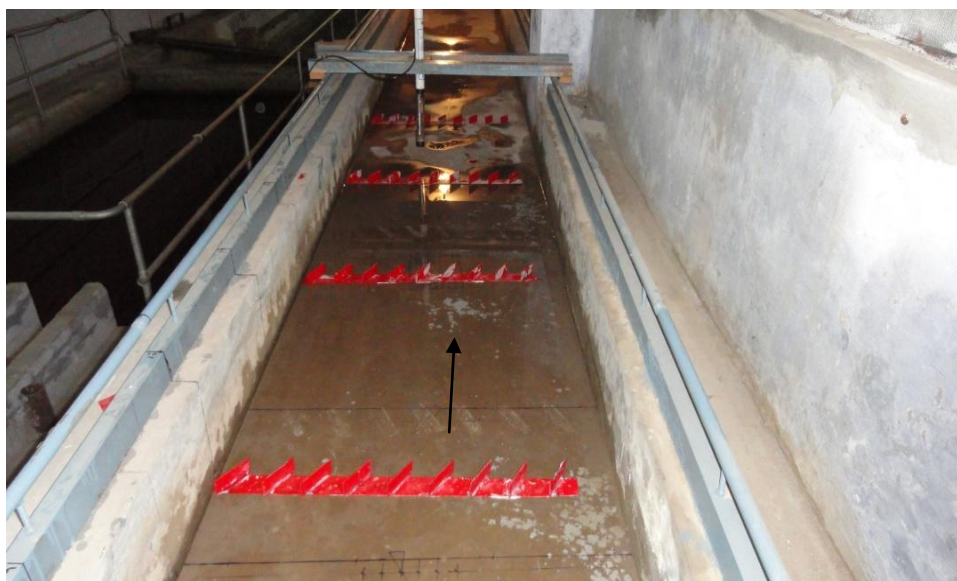
Figure 5. Four arrays of installed vanes
