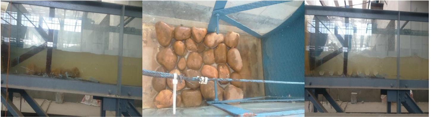
Figure 2. The different materials used downstream the radial gate.
