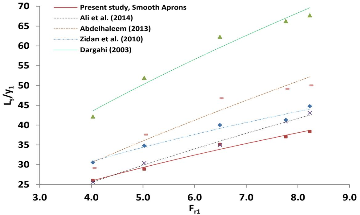
Figure 9. Relationship between  $(L_s/y_l)$  and  $Fr_1$  over smooth apron for the present study and previous research works.
