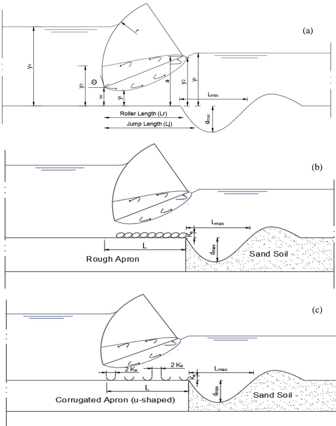
Figure 1. Layout of scour due to submerged jump on different aprons a) Smooth apron b) Rough Apron c) Corrugated Apron downstream radial gate.
