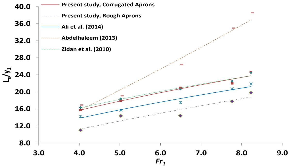
Figure 10. Relationship between  $(L_s/y_l)$  and  $Fr_1$  over corrugated and rough aprons for the present study and previous research works.
