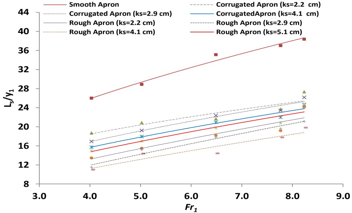
Figure 7. Relationship between observed relative scour length ( $L_s/y_1$ ) with  $Fr_1$  over smooth, corrugated and rough aprons at submergence factor  $S=0.4$
