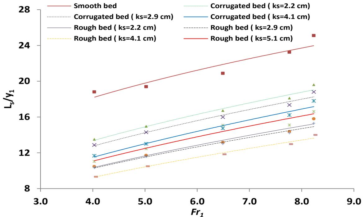
Figure 8. Relationship between observed relative scour length ( $L_s/y_1$ ) with  $Fr_1$  over smooth, corrugated and rough aprons at submergence factor  $S=0.1$
