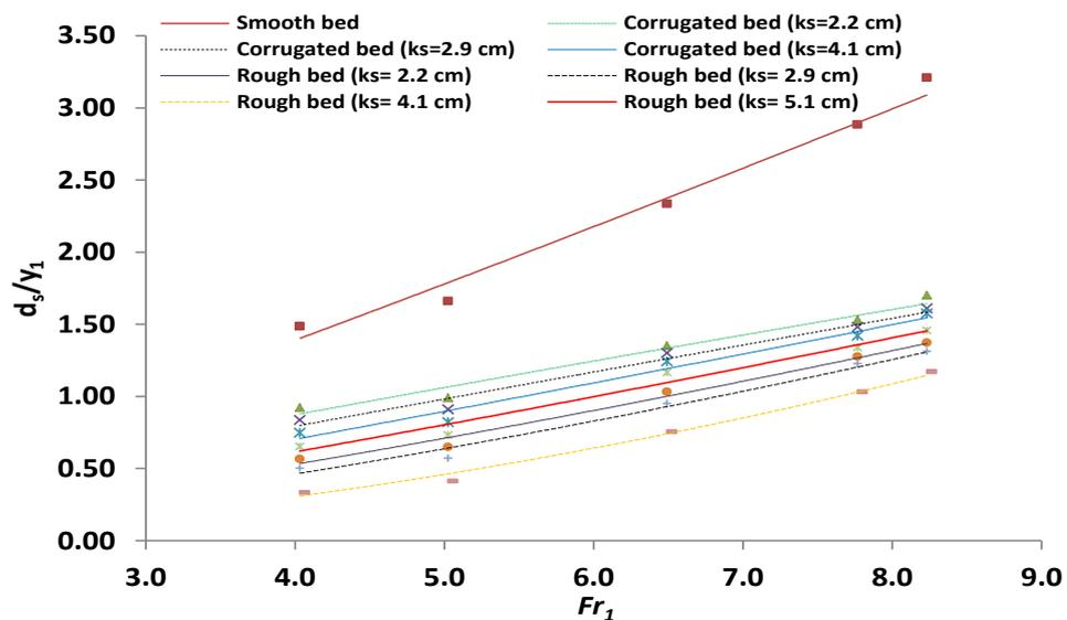
Figure 4. Relationship between observed relative scour depth ( $d_s/y_1$ ) with  $Fr_1$  over smooth, corrugated and rough aprons at submergence factor  $S = 0.1$
