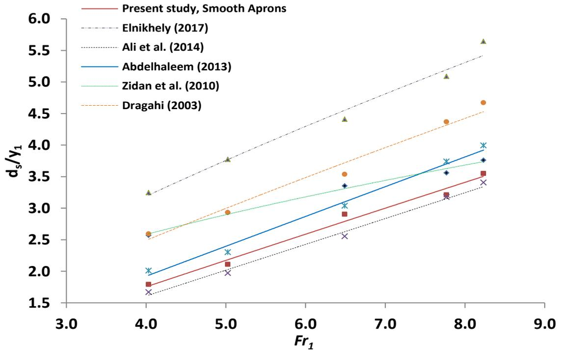
Figure 5. Relationship between  $(d_s/y_1)$  and  $Fr_1$  over smooth apron for the present study and previous research works.
