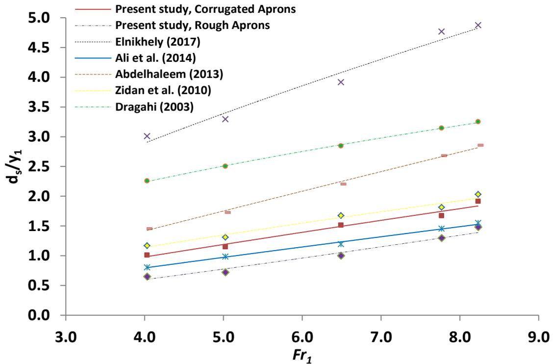
Figure 6. Relationship between  $(d_s/y_1)$  and  $Fr_1$  over corrugated and rough aprons for the present study and previous research works.
