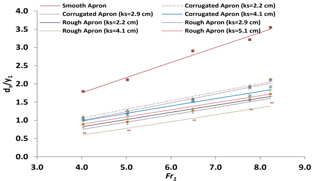
Figure 3. Relationship between observed relative scour depth ( $d_s/y_1$ ) with  $Fr_1$  over smooth, corrugated and rough aprons at submergence factor  $S = 0.4$
