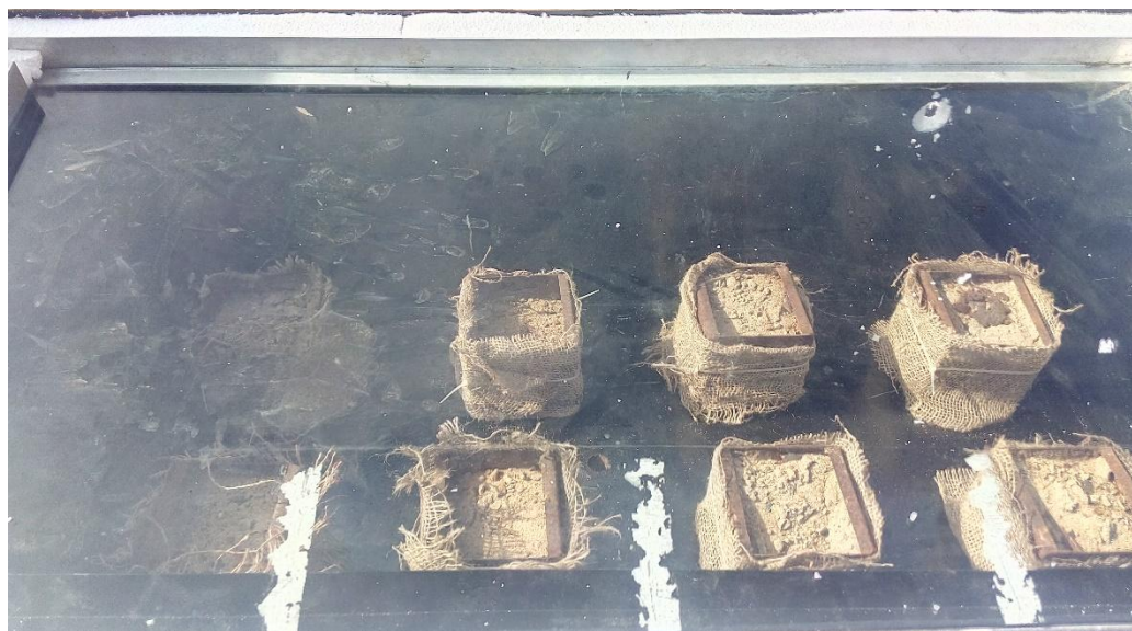
Figure 1. Experimental photograph of modified solar still with jute cloth knitted to sensible heat energy storage
