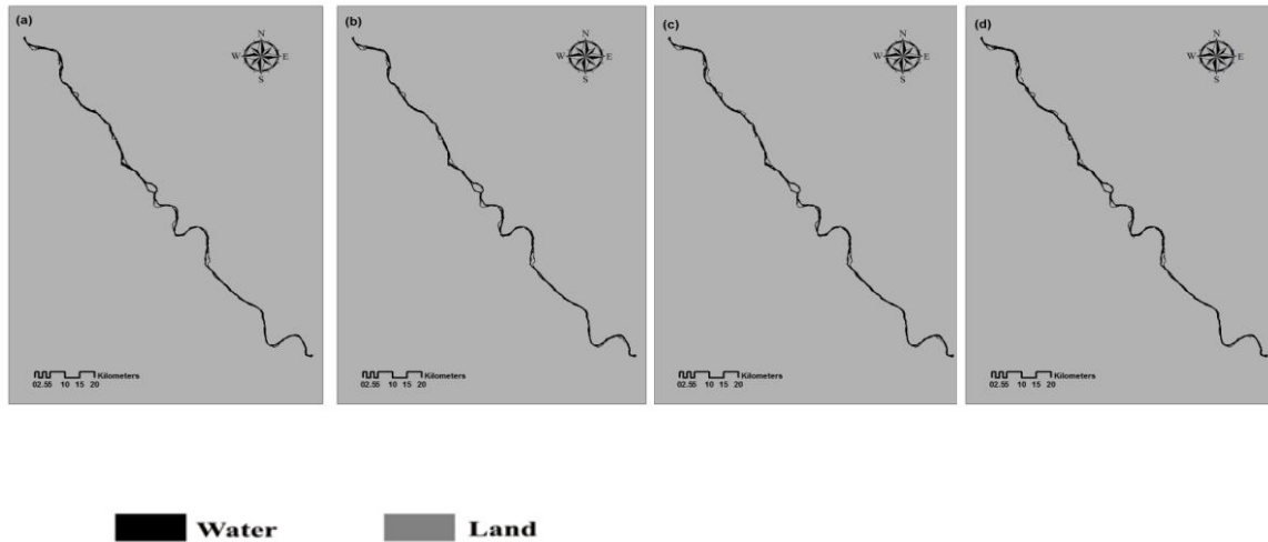
Figure 3. the extracted water surface maps from Landsat 5 TM image (2010).(a) Reference map; (b) NDWI map; (c) AWEI map; (d) WRI map.
