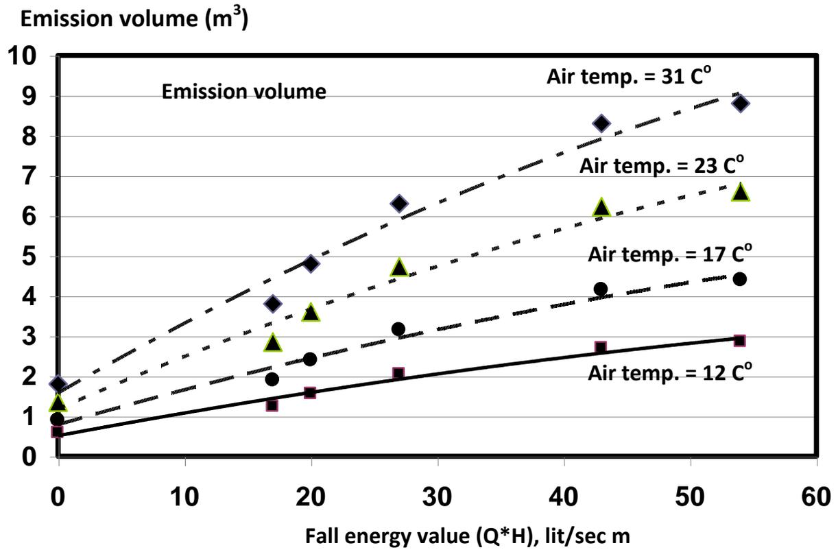
Figure 4.illustrates maximum gases volume inside manholes after two months against the fall energy value (Q\*H),
