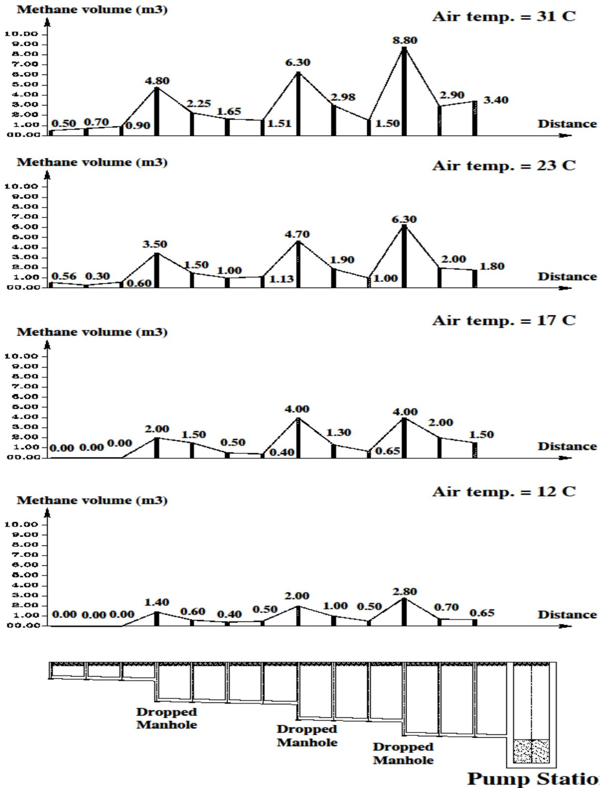
Figure 3. illustrates maximum gases volume inside manholes after two months during different seasons
