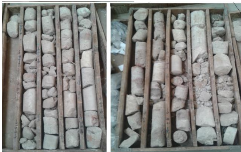
Figure 19. Core samples extracted from boring No. (1)
