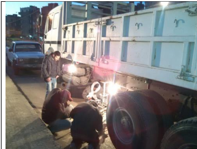
Figure 20. The used truck as a reaction frame on the top of one of the tested openings
