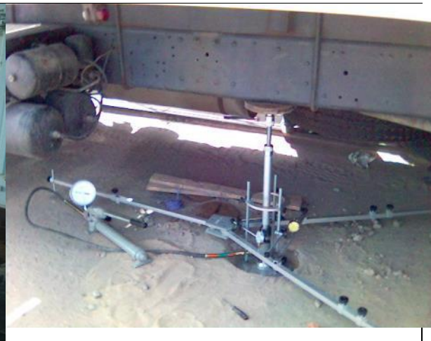
Figure 21. The used plate loading device during the test
