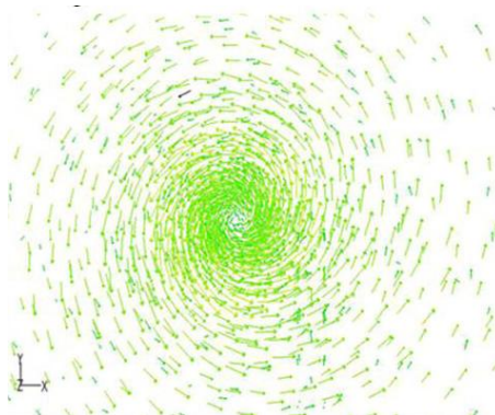
Figure 2.Velocity vectors of swirl flow dominates in the flocculation zone
