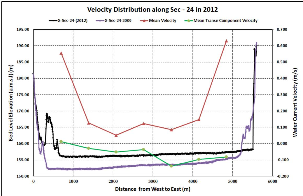
Figure 12 . Comparison of Mean Transverse Velocity with Channel Bed Morphological Changes at Sec - 24 in 2012.
