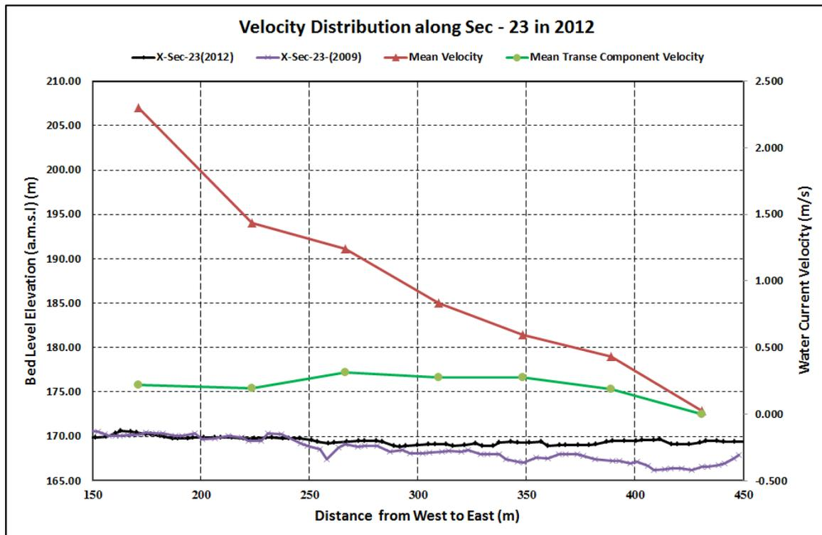
**Figure 6 . Comparison of Mean Transverse Velocity with Channel Bed Morpholgical Changes at Sec - 23 in 2012.**
