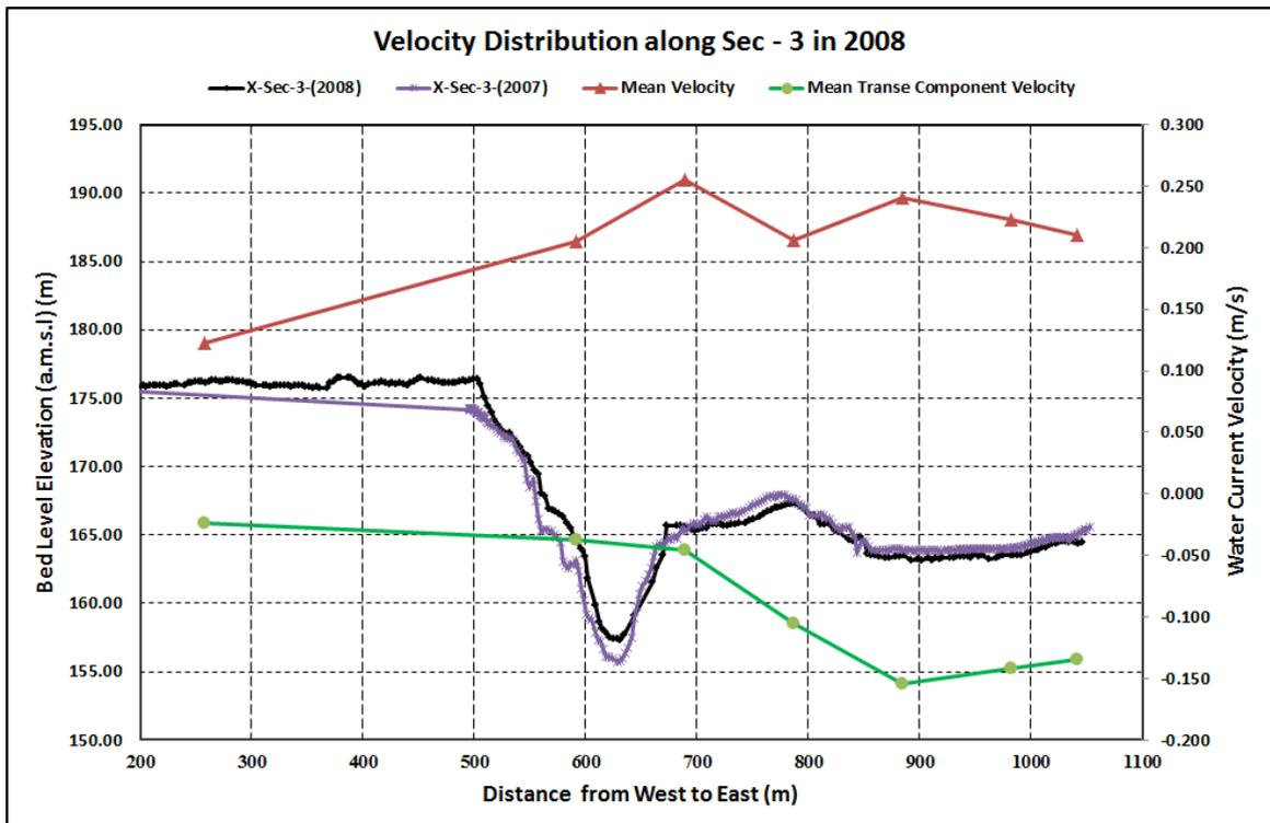
Figure 8 . Comparison of Mean Transverse Velocity with Channel Bed Morphological Changes at Sec - 3 in 2008.
