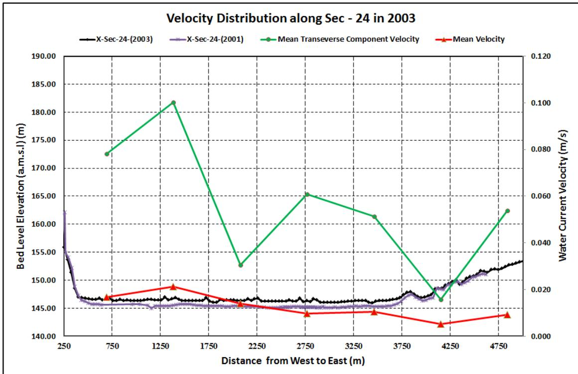
**Figure 10 . Comparison of Mean Transverse Velocity with Channel Bed Morphological Changes at Sec - 24 in 2003.**
