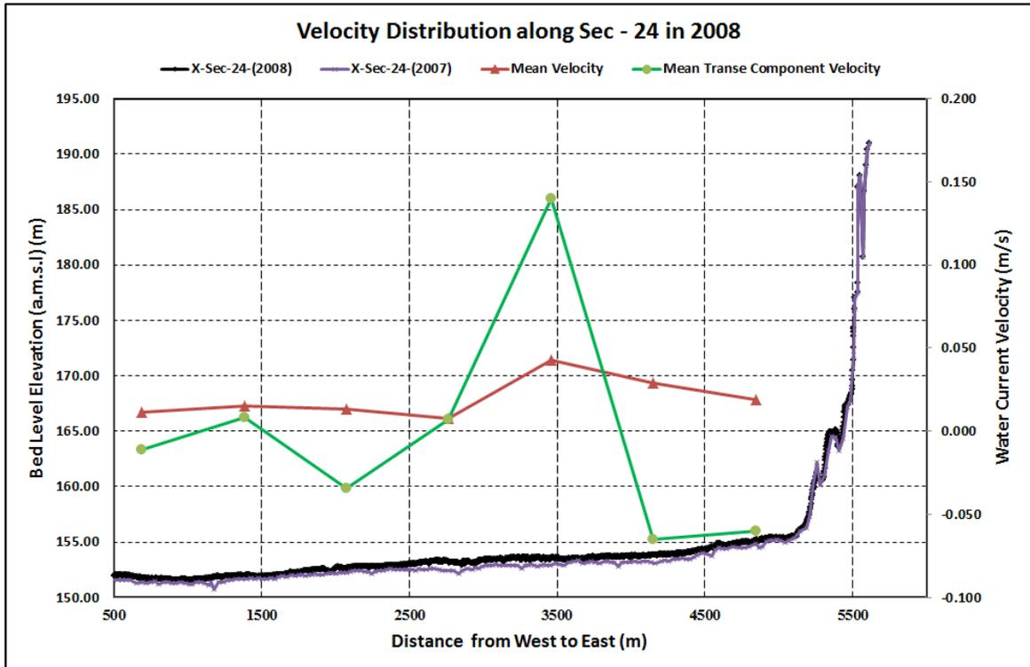
Figure 11 . Comparison of Mean Transverse Velocity with Channel Bed Morphological Changes at Sec - 24 in 2008.
