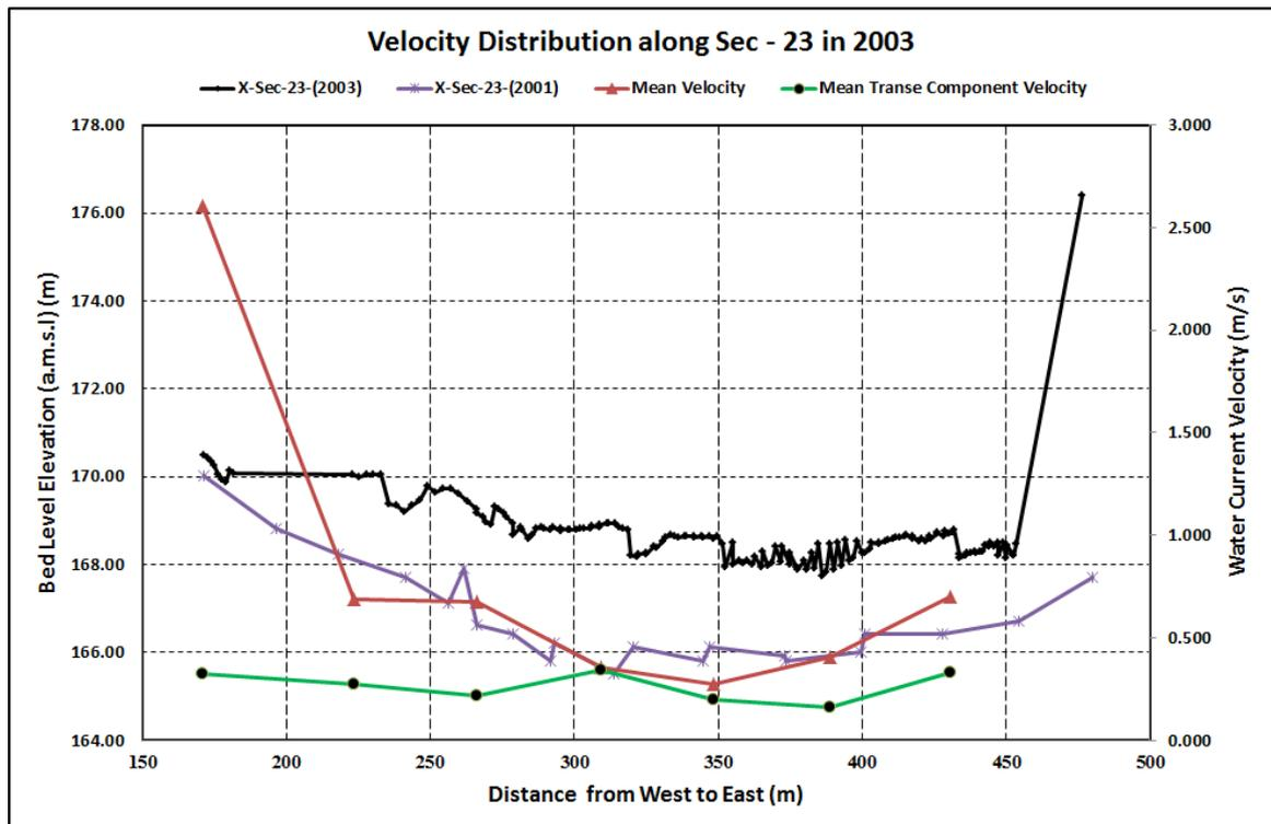
**Figure 4. Comparison of Mean Transverse Velocity with Channel Bed Morpholgical Changes at Sec - 23 in 2003.**
