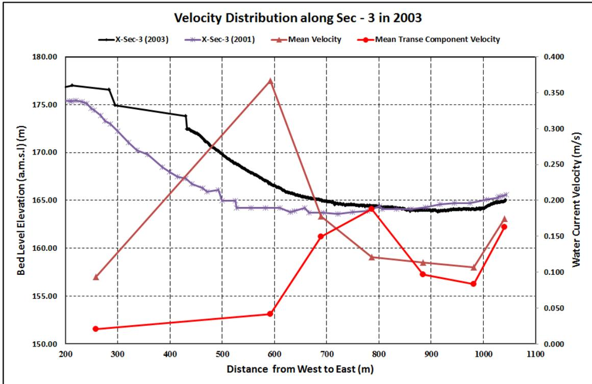
Figure 7. Comparison of Mean Transverse Velocity with Channel Bed Morphological Changes at Sec - 3 in 2003.
