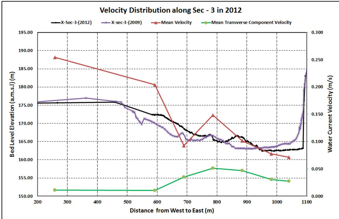
**Figure 9 . Comparison of Mean Transverse Velocity with Channel Bed Morphological Changes at Sec - 3 in 2012.**
