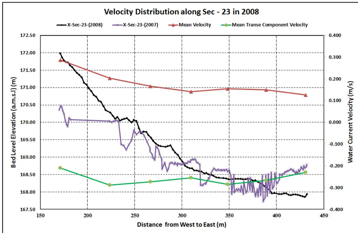
**Figure 5 . Comparison of Mean Transverse Velocity with Channel Bed Morpholgical Changes at Sec - 23 in 2008.**
