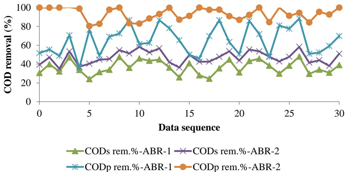
Figure 3b: Effect of maghemite nanoparticles on COD (soluble and particulate) removal efficiencies from starch wastewater industry
