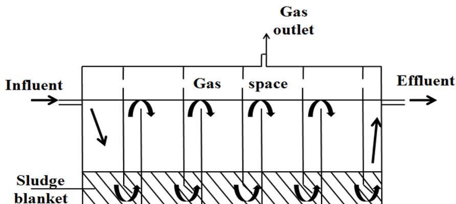
**Figure1: Schematic diagram of the anaerobic baffled reactor (ABR) treating starch wastewater industry**
