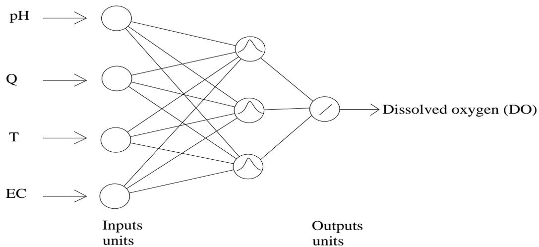
Fig. 2 Schematic diagram of RBNN architecture
