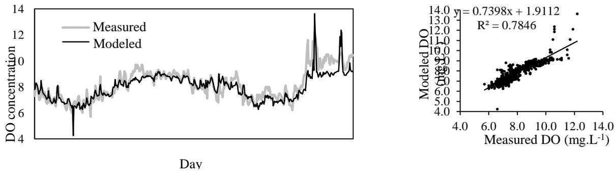
Fig. 4 Measured and modeled DO concentrations by ANFIS in validation phase
