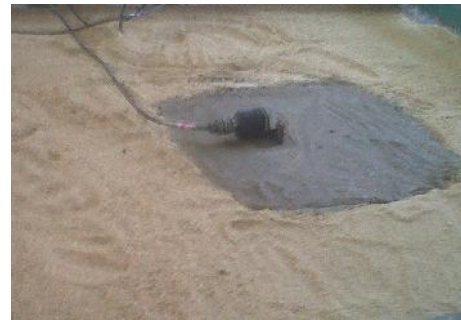
b) Accelerometer fixed at the grouted Area
