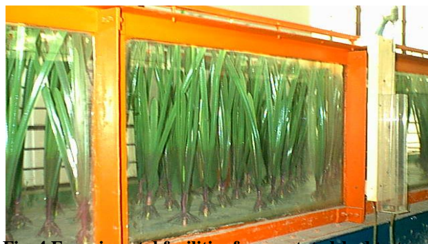
Fig. 4 Experimental facilities for vegetated-bed tests.
