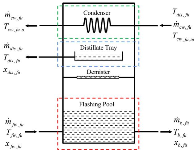
Fig. 7 Single stage flash desalination unit.
