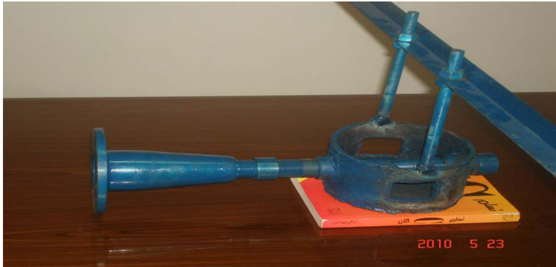
Fig. (3) Photo of the jet pump used in the experimental test rig
