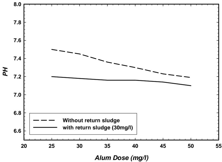
Figure 4 pH values with and without sludge dosing at different alum dosages
