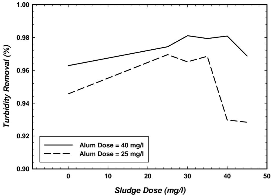
Figure 3 Turbidity removals at different sludge dosing with two different alum dosages
