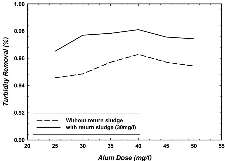
Figure 2 Turbidity removals with and without sludge dosing at different alum dosages
