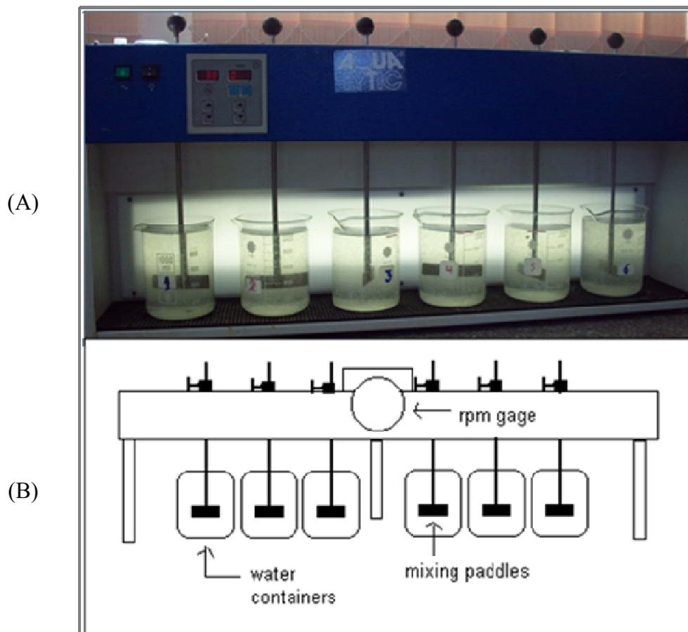
Figure 1 the laboratory floc tester: (A) photo, (B) schematic diagram
