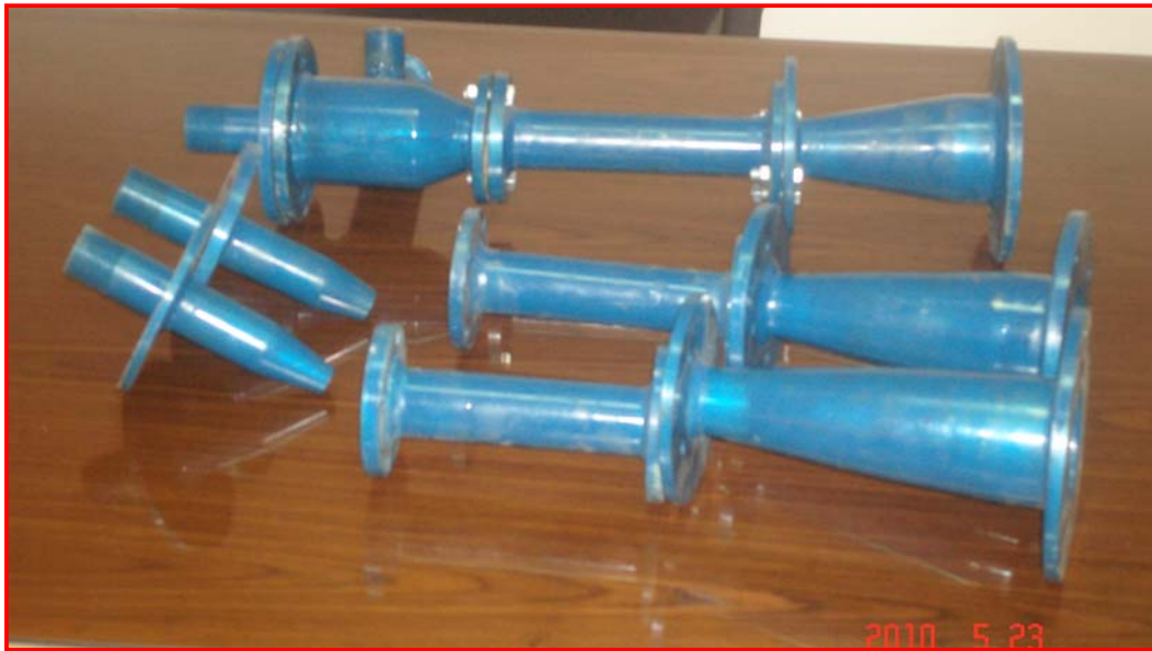
Fig.(3) Photo of the jet pump used in the experimental test rig
