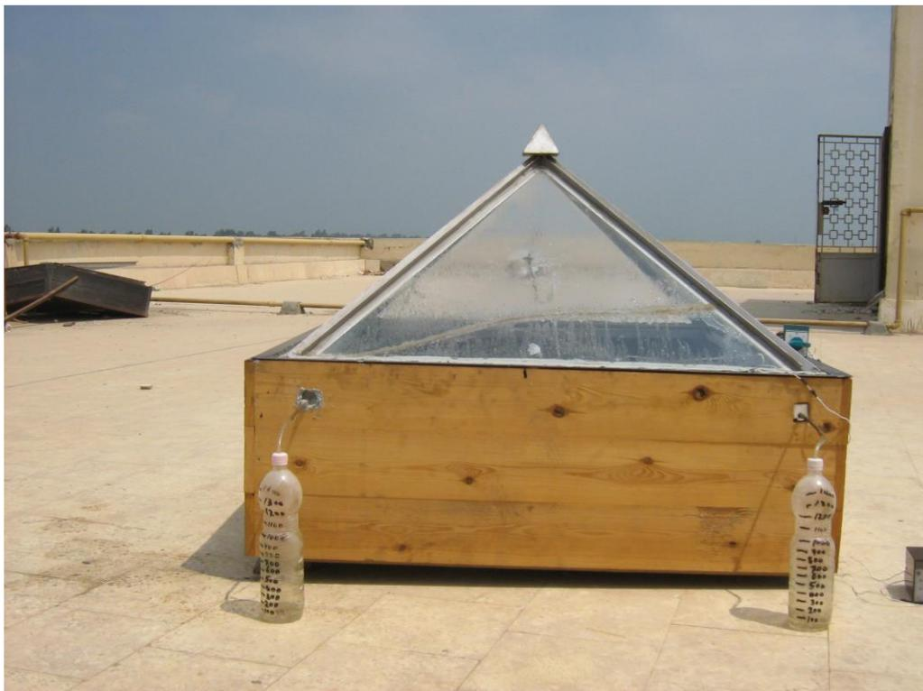
**Fig. 2. A photograph of the experimental solar still**
