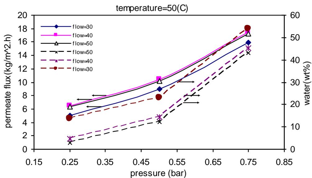
Figure 3 Effect of pressure on permeate flux and water content at different flow rates
