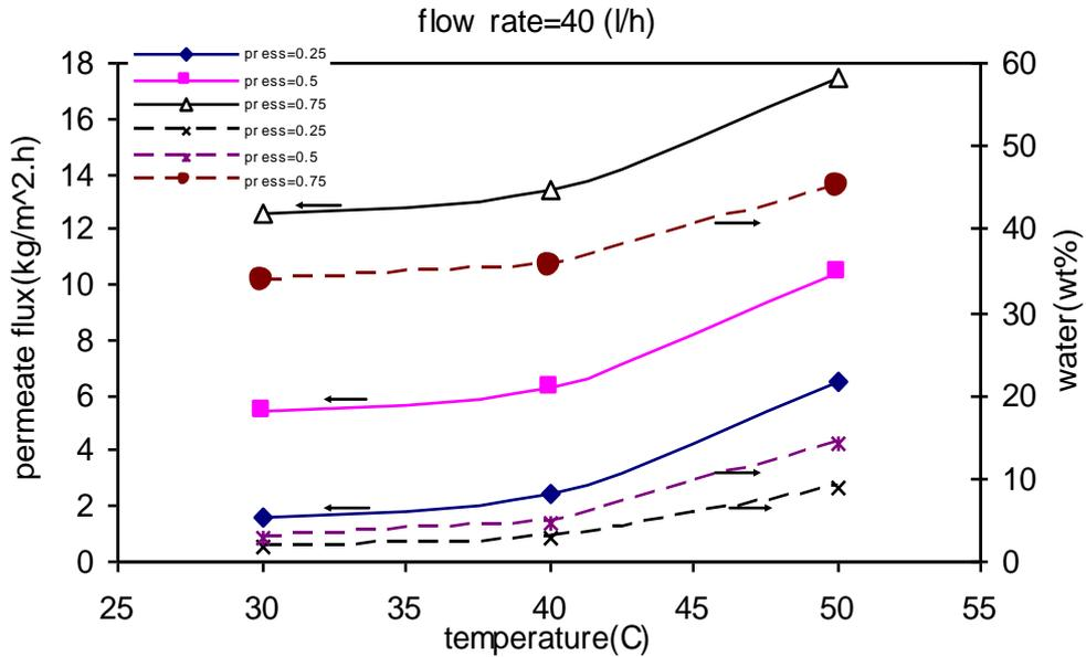
**Figure 5 Effect of temperature on permeate flux and water content at different pressures**
