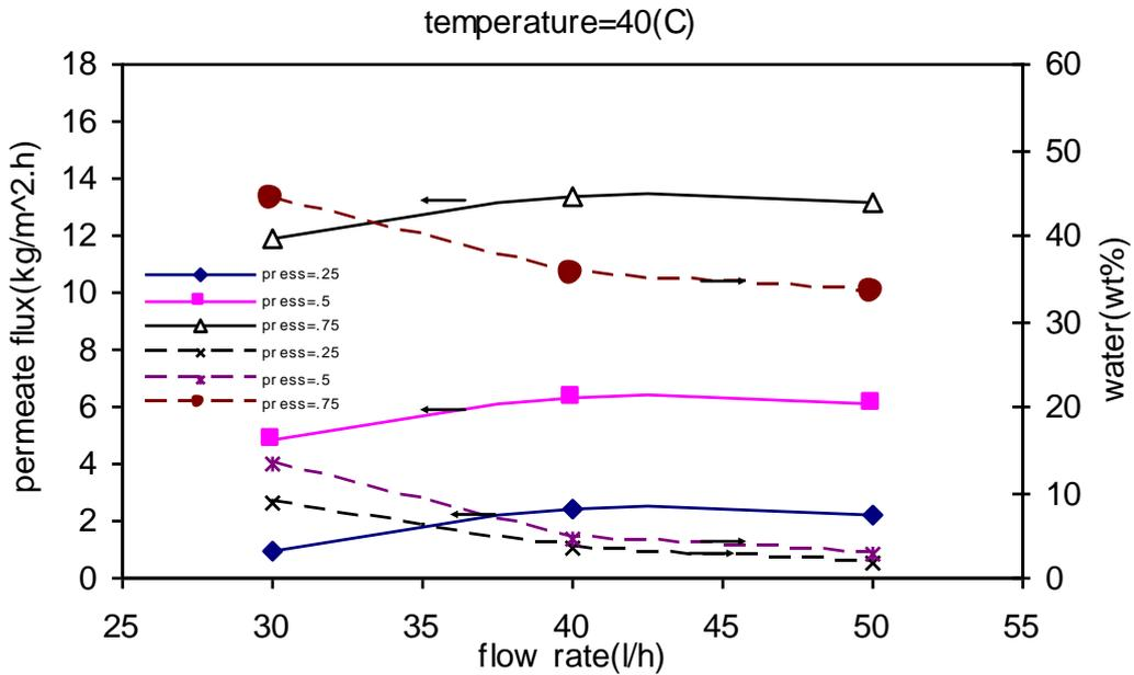
**Figure 7 Effect of flow rate on permeate flux and water content at different pressures**
