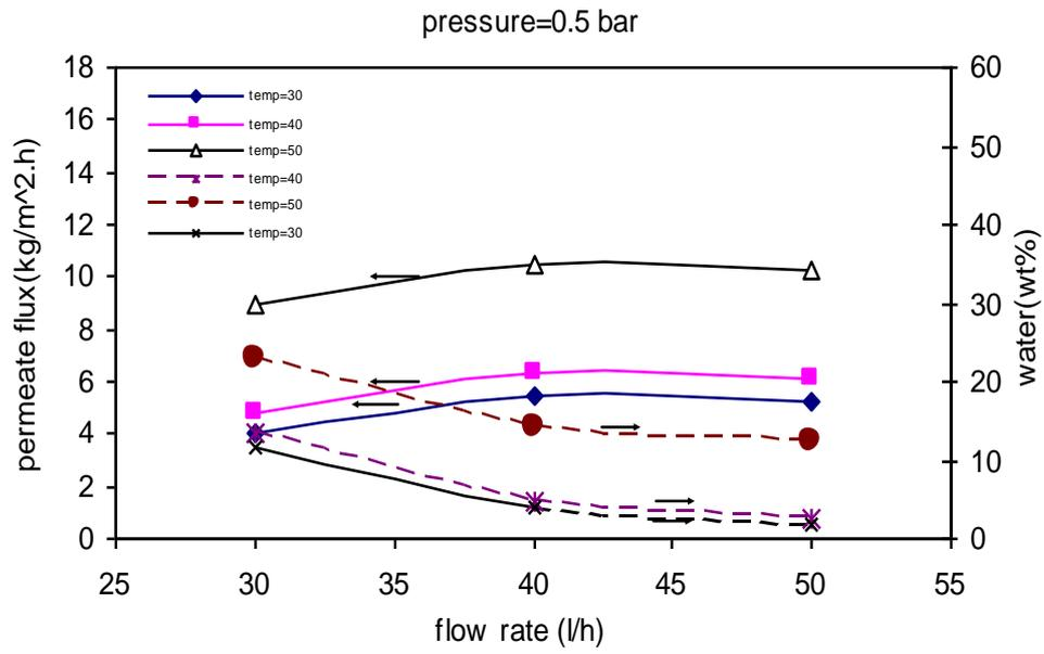
**Figure 8 Effect of flow rate on permeate flux and water content at different temperatures**
