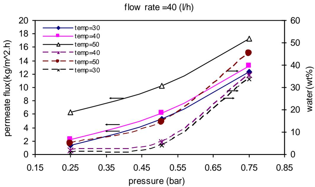
**Figure 4 Effect of pressure on permeate flux and water content at different temperatures**
