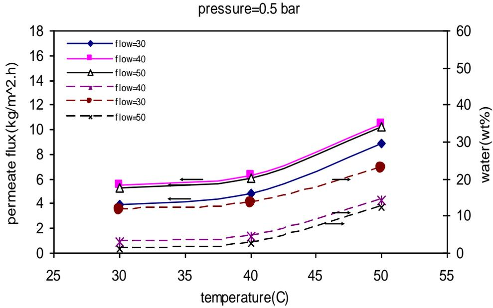
**Figure 6 Effect of temperature on permeate flux and water content at different flow rates**
