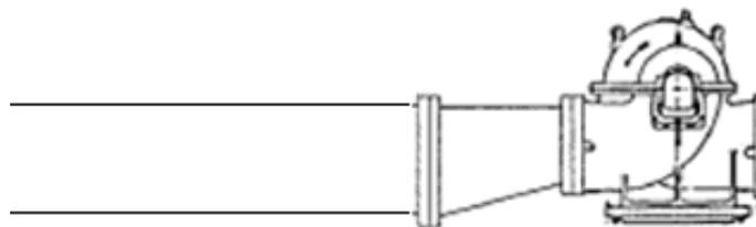
**Figure (6) Recommended suction pipe and reducer at the suction side**
