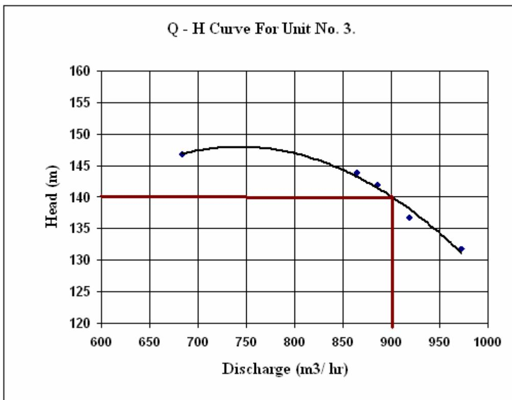
Figure (1). Hydraulic Performance Curve for Unit No. 3
