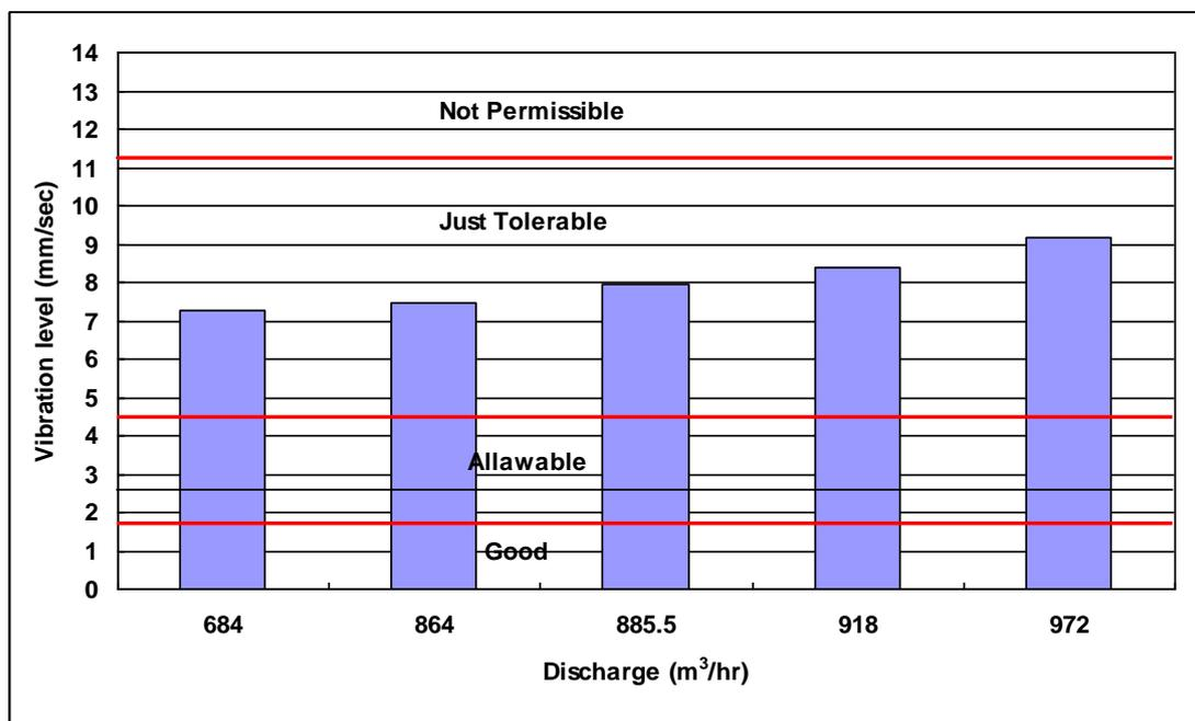
**Figure (2) Vibration levels measured within different pump capacity for unit No. 3 (according to ISO 2372 standard)**
