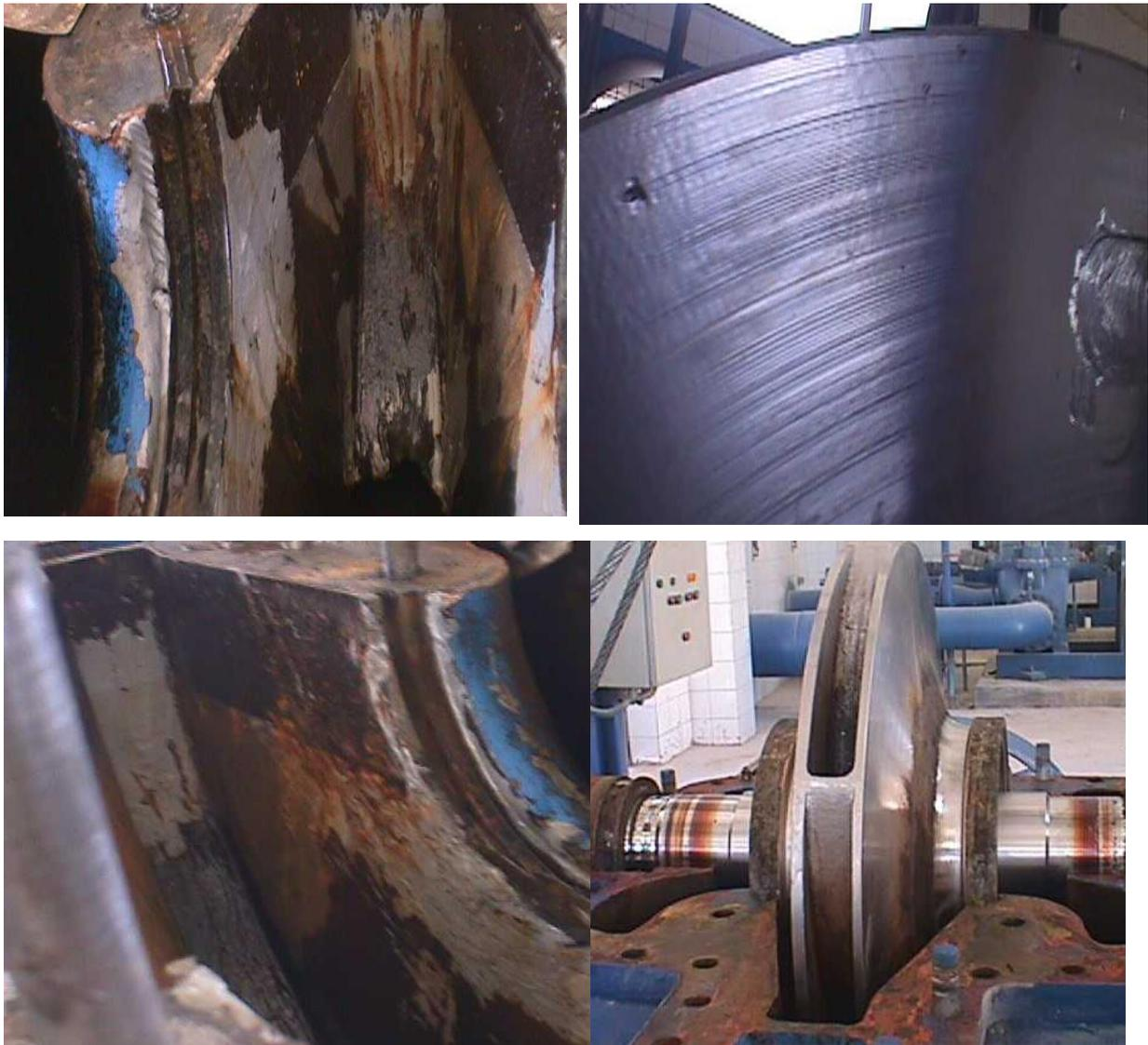
**Figure (4). Cavitation damage at the casing and pump impeller**
