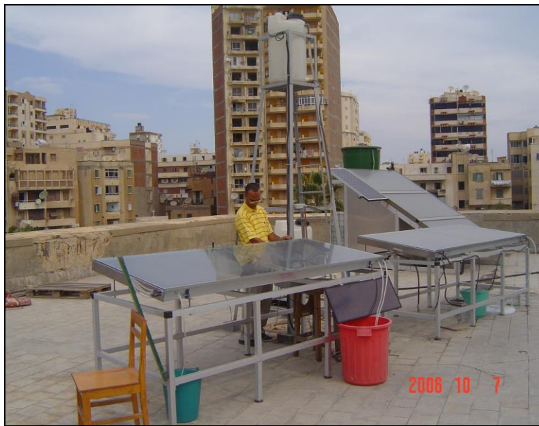
Figure (1) Testing and Improving still efficiency through the recovery of lost energy with product water and brine
