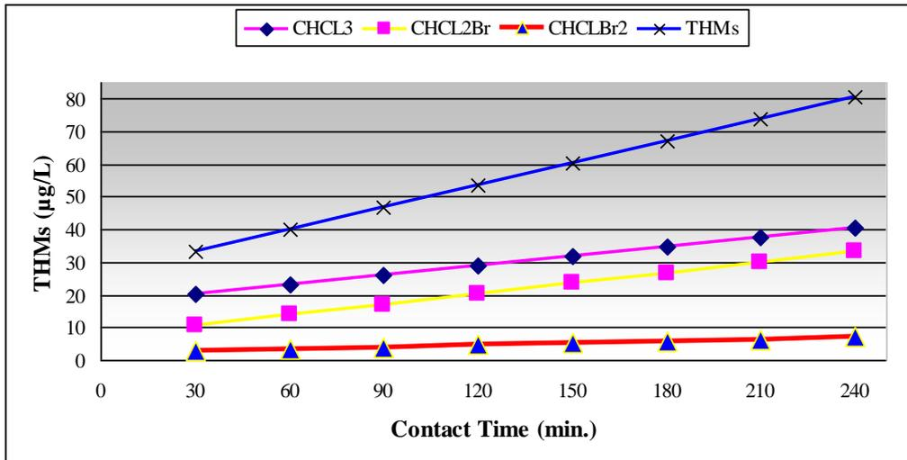
**Figure 3: Effect of Contact Time on THMs Formation** (6 mg/L of chlorine, at pH 7 and at room temperature)
