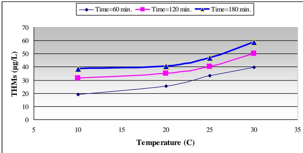
**Figure 5: Effect of Temperature on THMs Formation (6 mg/L of chlorine at pH 7)**
