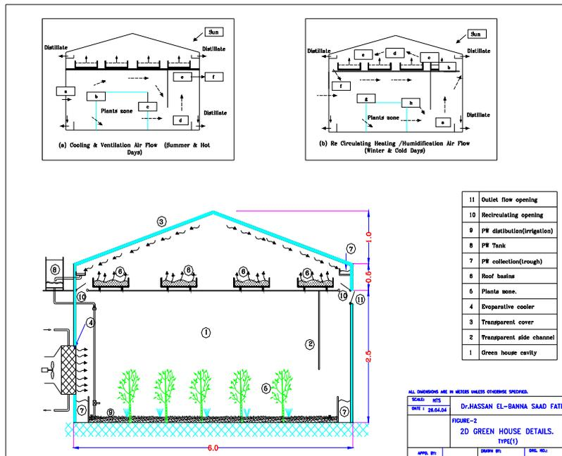
Fig (2) Type-1 GH with Roof Solar Basins
