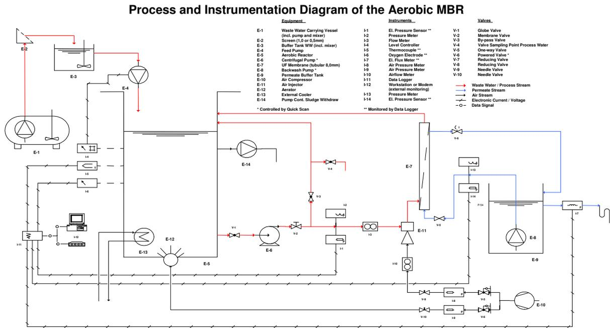
**Figure (A): Process scheme diagram of the aerobic side stream MBR system**
