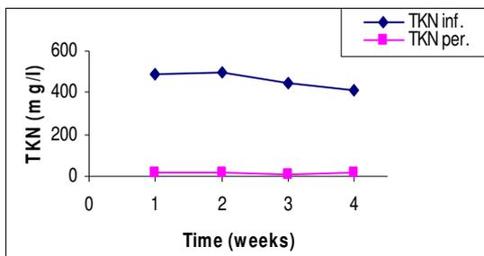
Fig 4: TKN values for potato-processing wastewater at HRT 24 hr and air flush: water ratio = 1:1.
