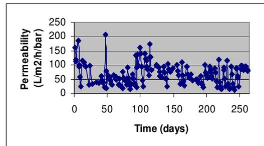
Fig 8: Permeability of the side stream MBR during the treatment of the potato-processing wastewater
