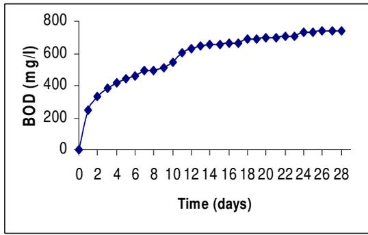
Fig 1: BOD biodegradability of the potato processing wastewater
