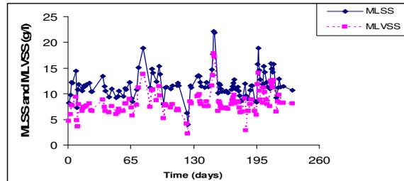
Fig 6: MLSS and MLVSS (g/l) of the side stream MBR during the treatment of potato processing wastewater
