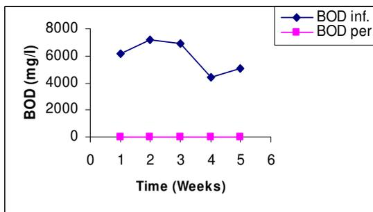
Fig 3: BOD values for potato-processing wastewater at HRT 24 hr and air flush: water ratio = 2:1.
