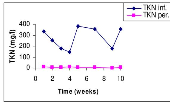
Fig 5: TKN values for potato-processing wastewater at HRT 24 hr and air flush: water ratio = 2:1.
