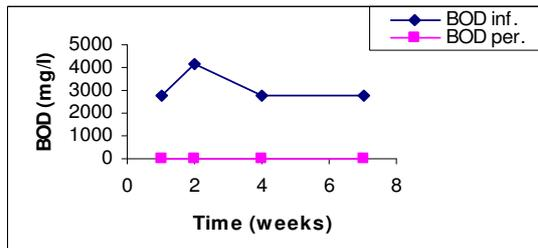
Fig 2: BOD values for potato-processing wastewater at HRT 24 hr and air flush: water ratio = 1:1.
