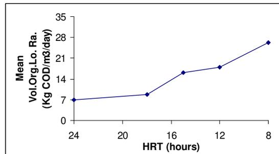
Fig 7: Mean Volumetric Organic Loading Rates at air flush: water ratio = 2:1 during the treatment of the potato-processing wastewater
