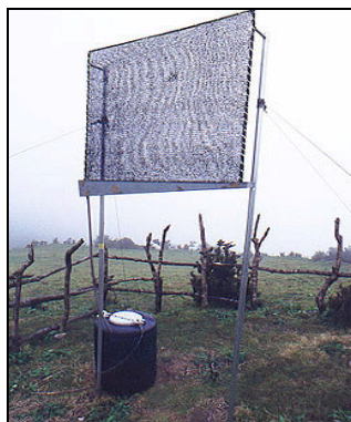
Figure 2-1: Actual SFC unit Photo: Keith Mac Quarrie
